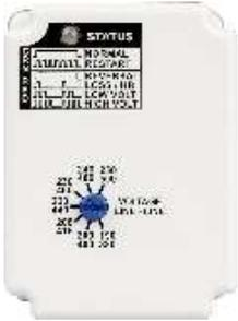
The Voltage Line-Line knob on the PMPU-FA8 has two ranges (left): a 190-250V low voltage scale and a 380-500V high voltage scale. The unit auto senses the 3-phase line-line voltage when applied and automatically selects the appropriate range.
