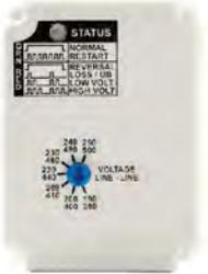
The Voltage Line-Line knob on the PMPU-FA8X & PMPU-FA12X has two ranges (left): a 190-250V low voltage scale and a 380-500V high voltage scale. The unit auto senses the 3-phase line-line voltage when applied and automatically selects the appropriate range.
