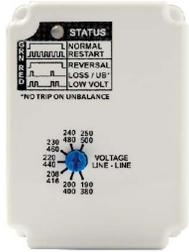
The Voltage Line-Line knob on the PJPU-FA8X has two ranges (left): a 190-250V low voltage scale and a 350-500V high voltage scale. The unit auto senses the three-phase line-line voltage when applied and automatically selects the appropriate range.
